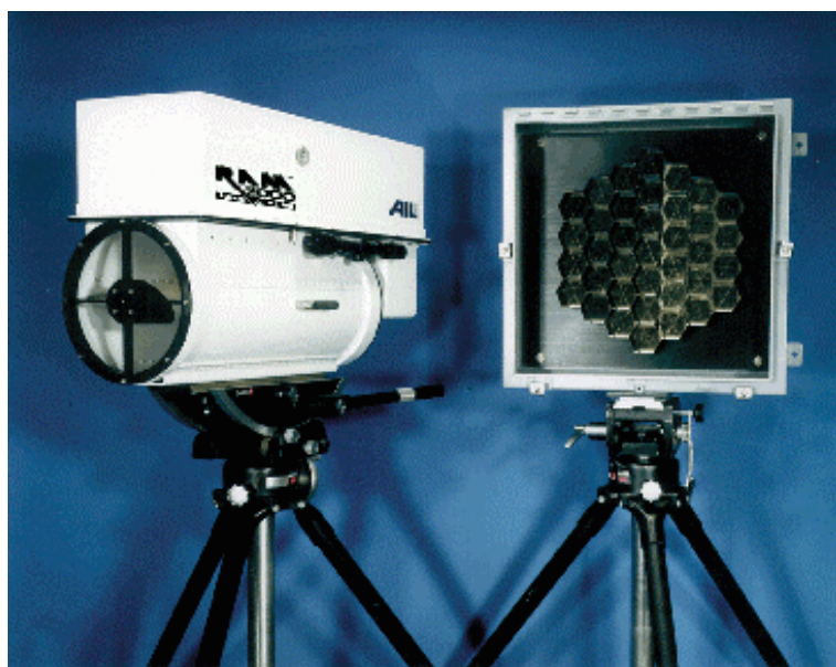
Figure 2-1. AIL RAM 2000 FTIR Optical Open-Path Monitor and Retroreflector
